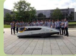
The solar cells of Stella generate more electricity on average than the car uses, meaning the surplus electricity can be returned to the power grid, making the car 'energy-positive'.
